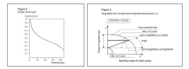
The proper selection of regulated pumps is shown in figures 3, 4 and 5. (Comparison of pump's characteristics determined by the design with actual technical characteristics of a particular pump).
