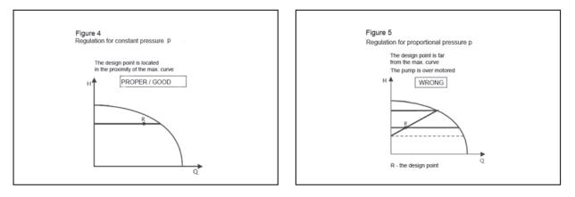
While using regulated pumps you can benefit from the operational field of a particular pump, which ranges from the minimal to the maximal Q-H curves. That is why such a regulation type is called stepless thermal regulation. The R design point should be located as close as possible to the functional max. Q-H curve.
